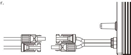
Figure Connect the DC connector
